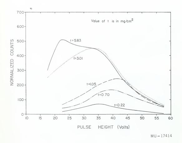
Fig. 4. Experimental differential pulse-height spectra with spallation-produced pulses subtracted.
